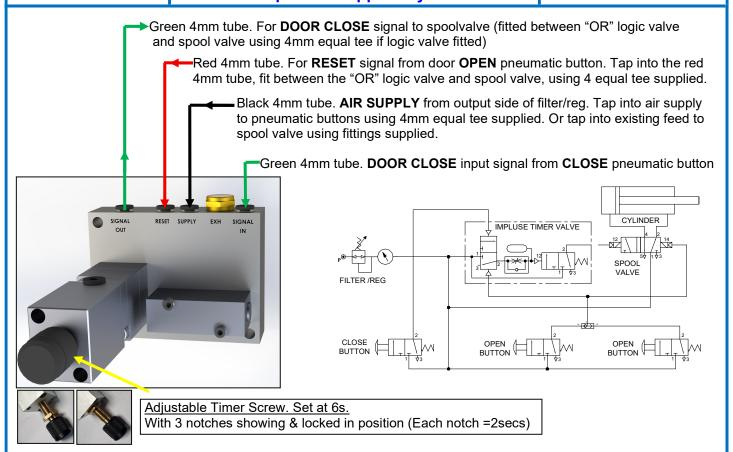
Spec:  $(2 \rightarrow 10 \text{bar})$  (  $1 \rightarrow 10 \text{s}$  Pneumatic Timer) (Temp,  $-20 \rightarrow +80^{\circ}\text{C}$ ) (Ports 4mm Push in type) Fitted between a trip valve (pneumatic button) and directional control valve (spool valve) for a pressure applied system.
